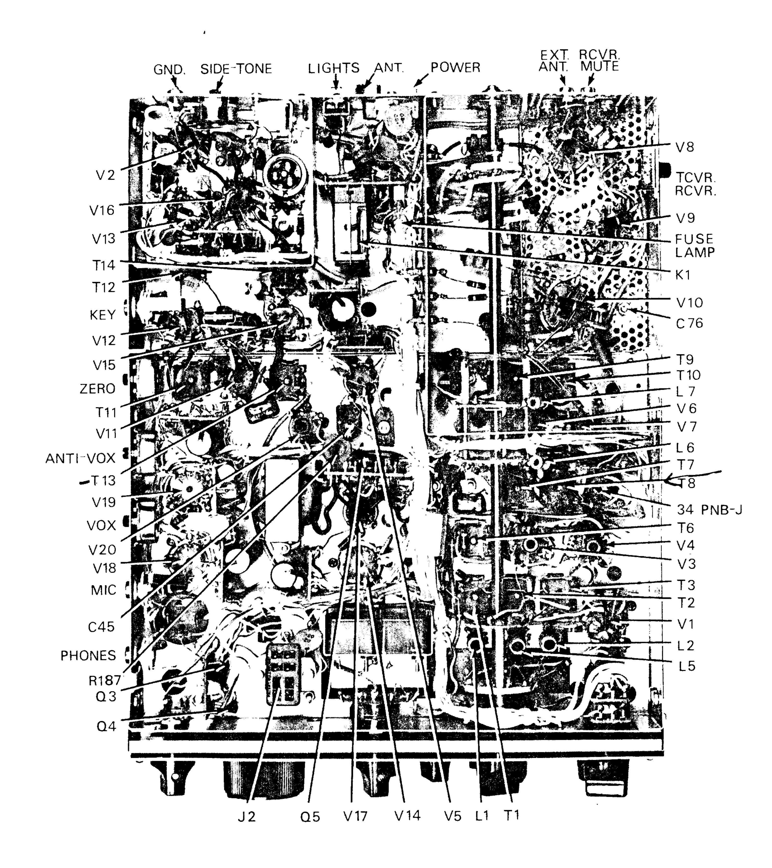
Figure 5-2. Alignment Locations, Bottom View
