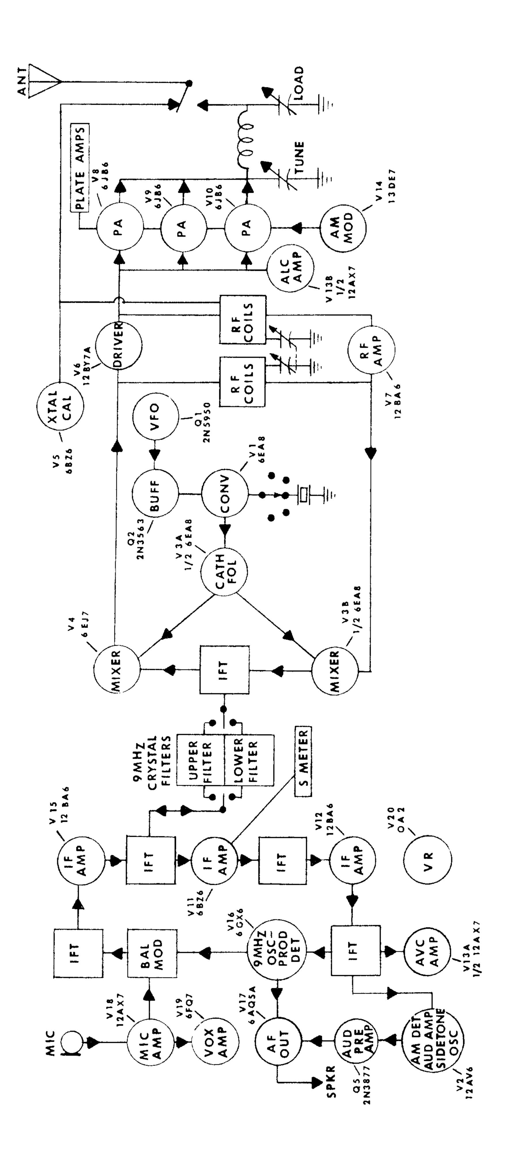
Figure 4-1. Block Diagram
