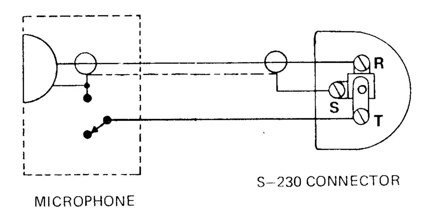
Figure 2-1. Microphone Connections
