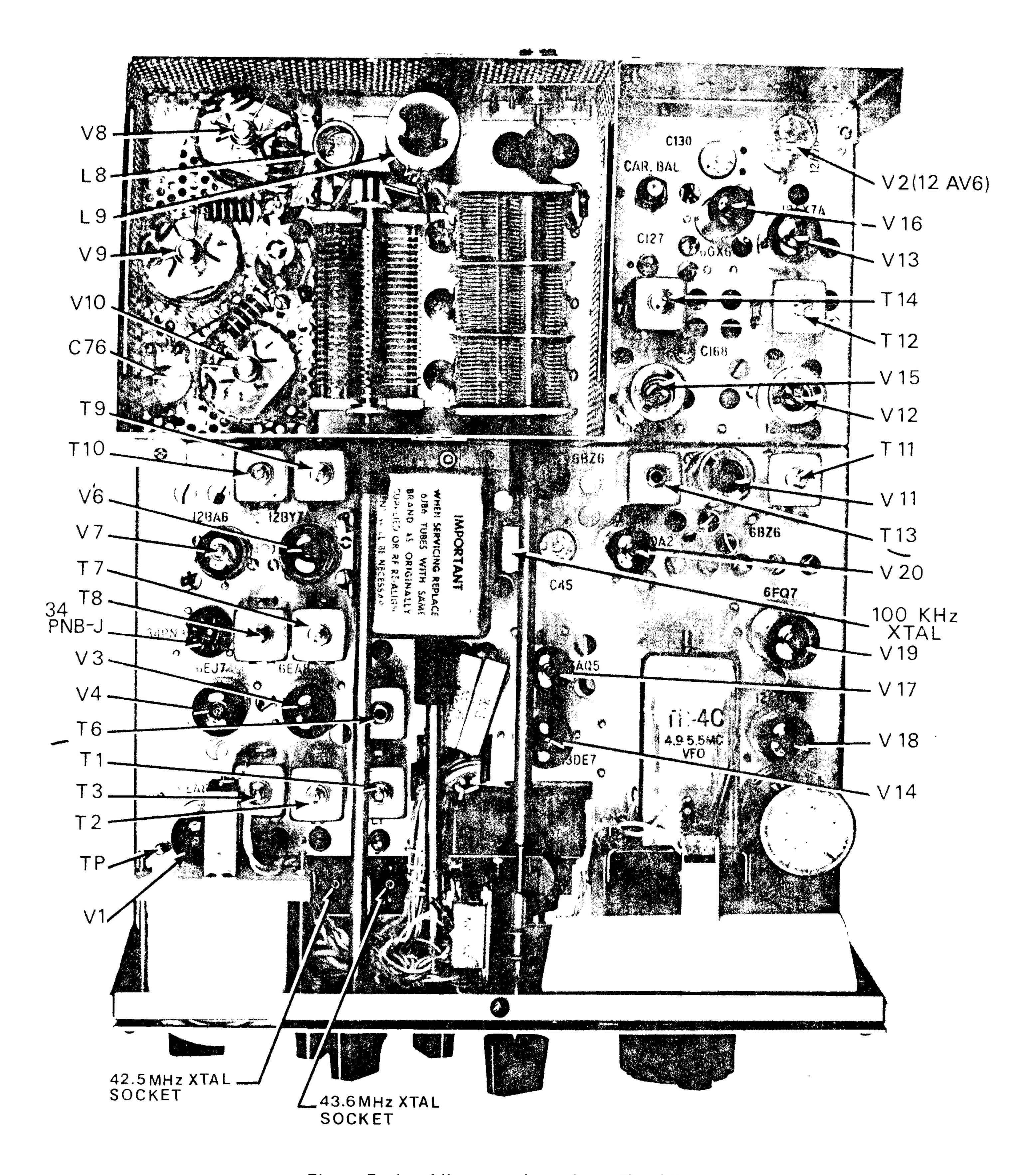
Figure 5-1. Alignment Locations, Top View
