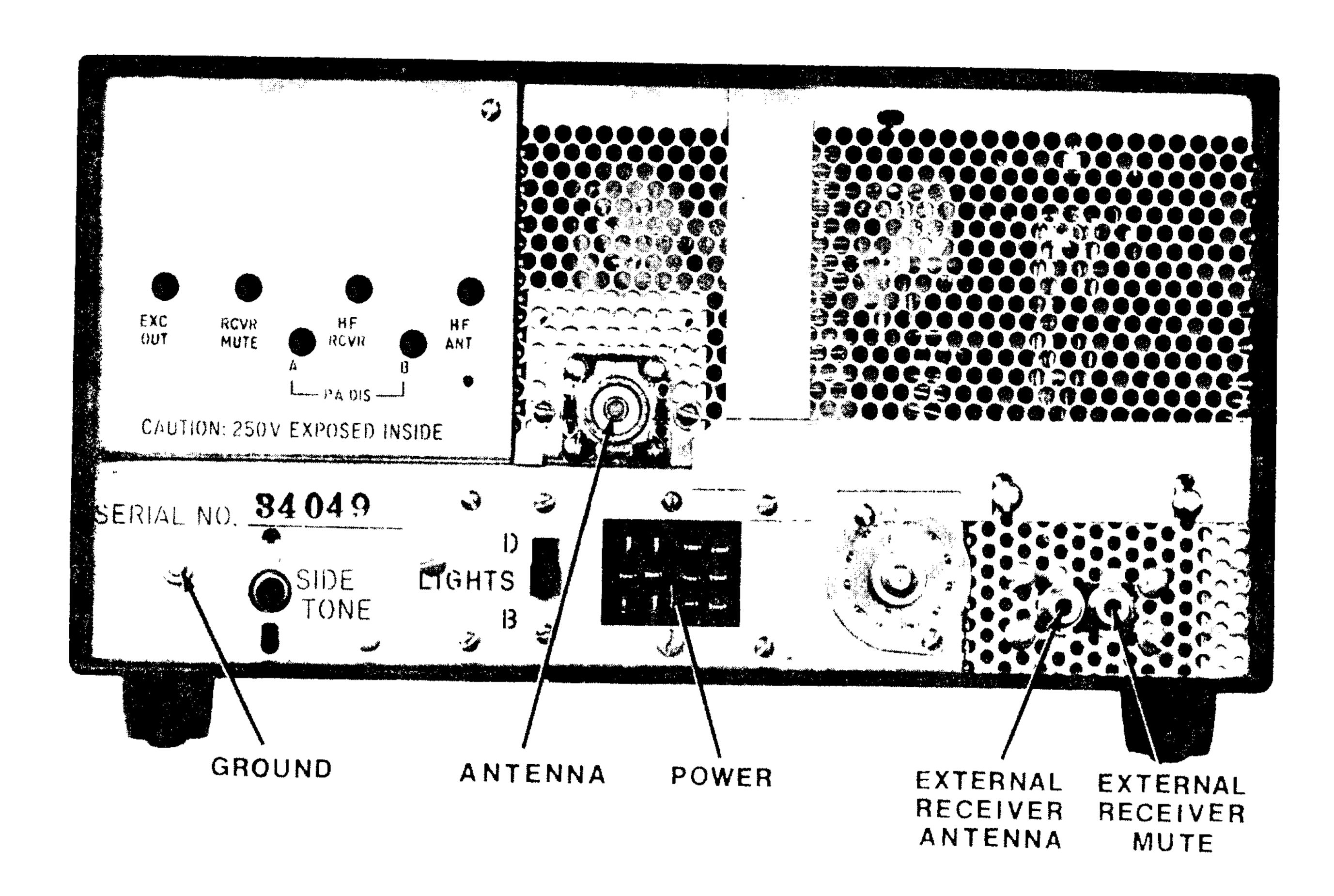
Figure 2-2. Rear Chassis Connectors
