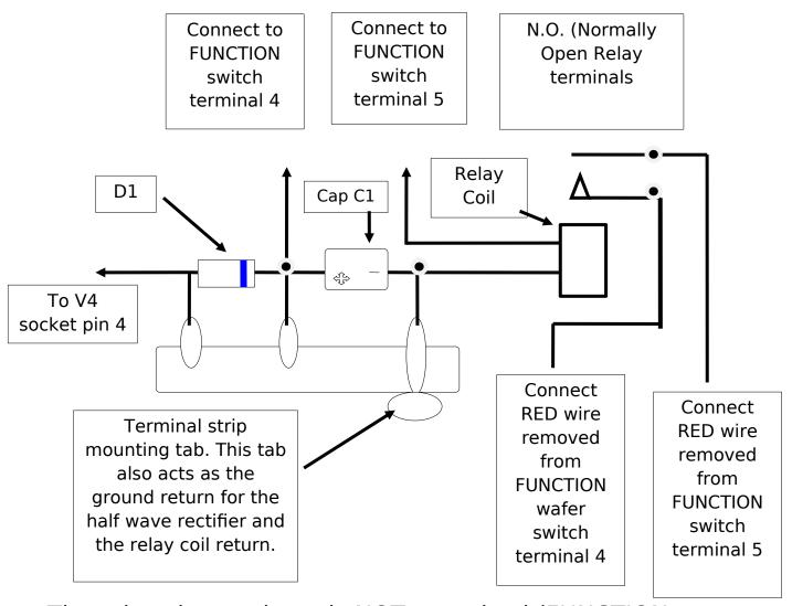
The relay shown above is NOT energized (FUNCTION switch set to OFF or STANDBY). The relay energizes in "TUNE, PHONE, and CW" positions only.
