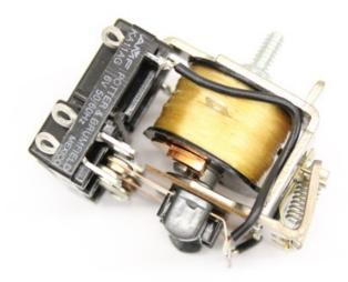
I use a rubber grommet slid over the threaded stud between the relay and the chassis to reduce the noise created when the relay energizes (click sound). A hole is drilled into the chassis to mount the relay below the chassis.
