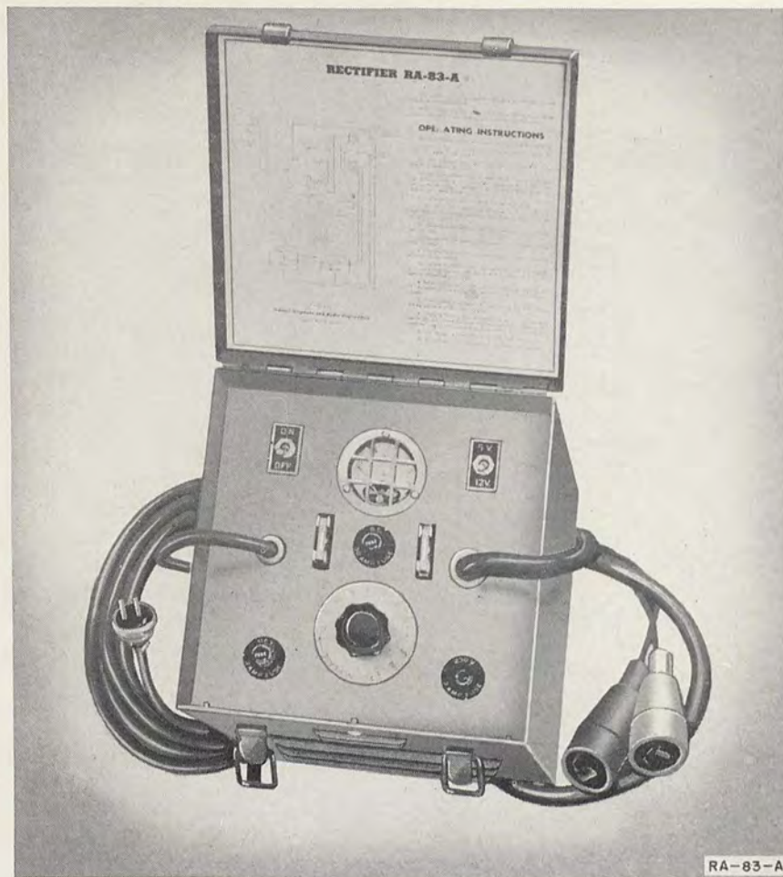
Figure 63. Rectifier RA-83-A, top view with cover open.
