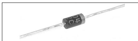
1N4004 diode. Band identifies cathode, or (+) end.
