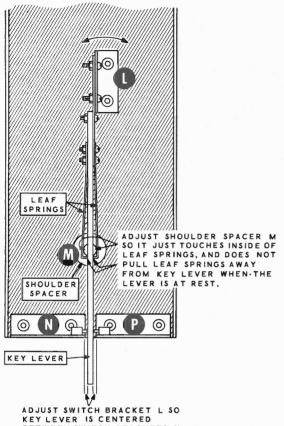
KEY LEVER IS CENTERED BETWEEN SWITCH BRACKETS N AND P.
