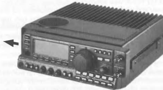
Installing the Front Sub-Panel
