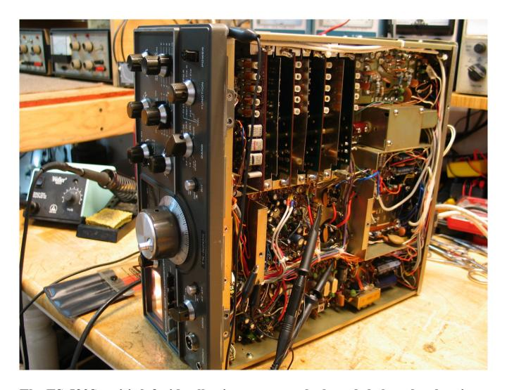
The TS-520S on it's left side allowing access to the boards below the chassis. Note the HV filter capacitor terminals are VERY CLOSE to the CAR and GENERATOR board connections. Use CAUTION when making and removing the scope probe connections.
