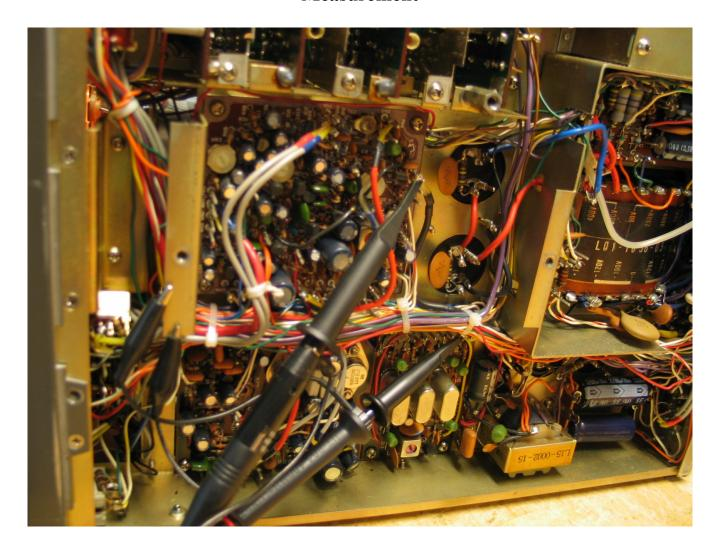
The top probe connects to the GENERATOR board "CAR" terminal. The bottom probe connects to the CAR board's "OUT" terminal. The 2 boards are accessible below the chassis as shown in the picture below. The 2 probes are connected to a dual trace scope not shown in the picture.
