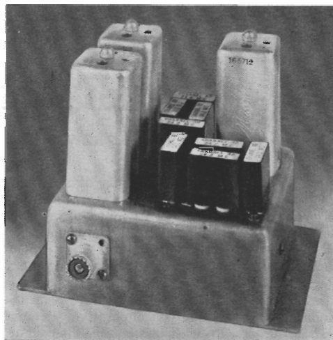
An experimental crystal lattice filter for receivers using surplus crystals. Its attenuation characteristic is shown in Fig. 5.
