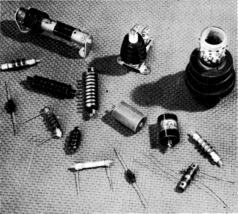
Fig. 304—This group of high-frequency (r.f.) inductors includes both transformers and chokes.
